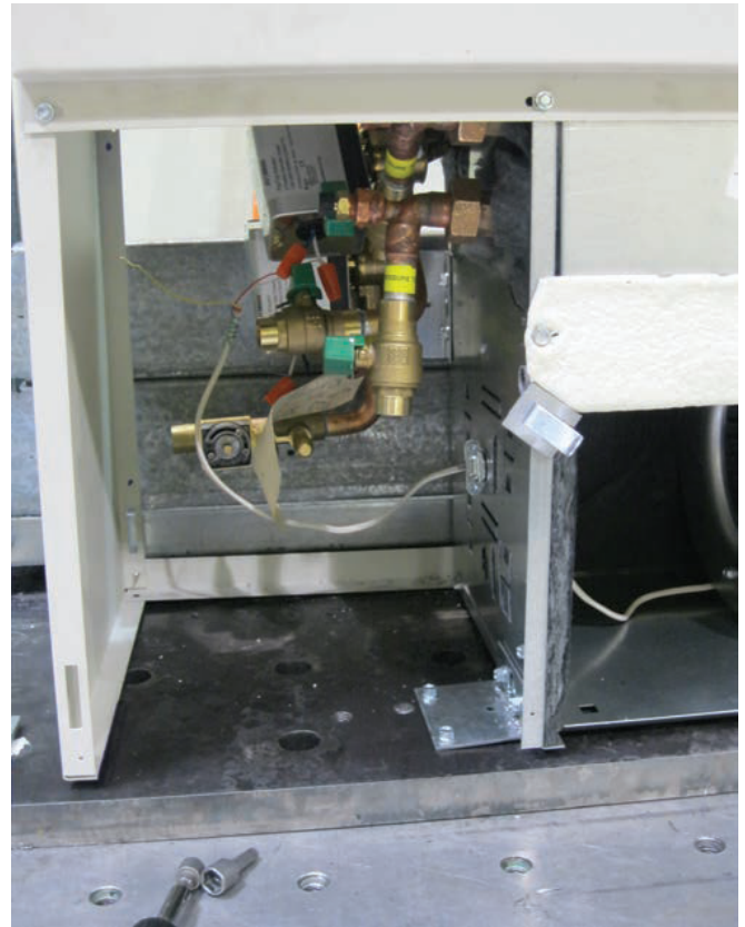
FIGURE 9 - FRONT CLIPS ATTACHED TO UNPAINTED SHEET-METAL FRAME
